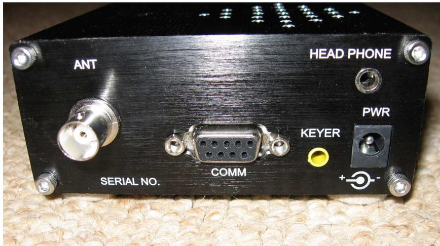
The power jack is a standard 5.5 x 2.1 mm jack coaxial power jack. The center pin is the positive connection, and the outer shell is the negative connection. Connect the radio to a suitable power source of 9.6 to 14.5 volts, direct current.
