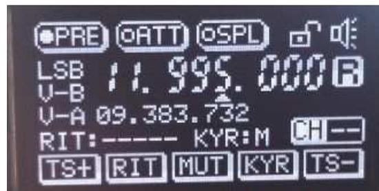
**RIT:** Receiver incremental tuning on/off. If on, set with frequency knob. Normal frequency setting is inhibited.
