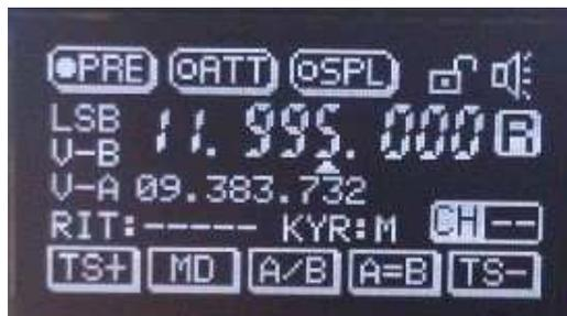
**TS+:** Frequency Step up. Underline shows digit that can be changed.
