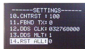
Rotate the frequency knob to select the desired menu item. Press the knob again to allow alteration of the value. Use the frequency knob and F1/F5 keys to select the desired digit. When you are done, press LK/SYS again for a “Yes – No” to save or not save the settings. Use the frequency knob to select “Yes” or “No.” Press the frequency knob to make your selection and return to normal operation.
